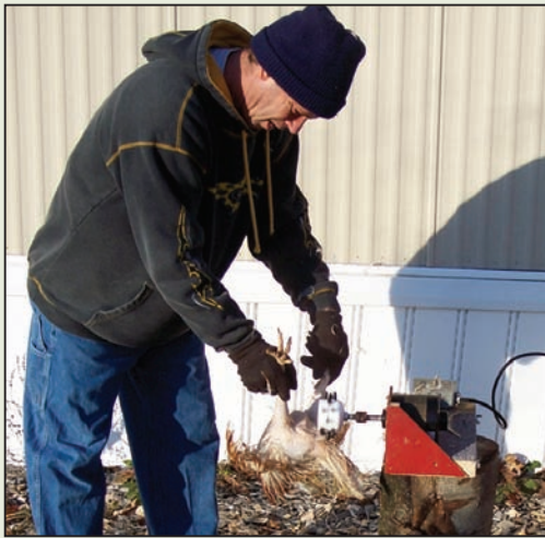
This small-scale chicken plucker can be made for about $10, using recycled materials.
