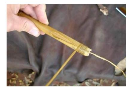
...when you're almost to the end of the sinew, slip a small loop of sinew (a separate piece that you prepared and set aside before starting to wrap) under the running end, and continue to wrap over that as well. In a second or two, you'll be using that loop to pull the running end back under itself.
