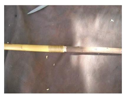
Here's a shot showing a perfect fit. The foreshaft is about 1/4" from its final position. For the moment, it's in as far as it will go using the pressure of my hands to push it in. The alignment looks good, and it's time to drive it in that last little bit by slamming it against a hard surface.
