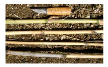
You can find ample amounts of material that is cured sufficiently for immediate use. The top piece is a little too green (although with some curing time - a few months, as it looses moisture slowly - it will be perfect). The second and third pieces from the top are perfect, and ready to be made into darts. The grey patches on the bottom piece tell me that it's a little to old and dry for an optimal dart. It will work, but it is more likely to break in use.
