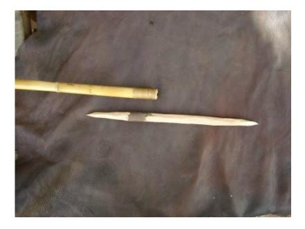
I've removed the fore-shaft by wiggling it back and forth a bit and carved it into a proper point. I left a bit of the bark on the fore-shaft to identify the thickest part. Again, the fore-shaft diameter is greater than the main shaft, and this prevents it from ever being forced inside to split the shaft.
