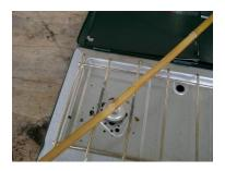
I've taken to using a camp stove as a heat source when straightening the cane. You want to avoid over heating the cane. When it's ready to bend, the outer rind will become glossy with "sweat" as the heat drives the moisture out of the cane. In the photo, you'll see a bit of a glossy shine right in the area over the heat source. This piece is ready to go..
