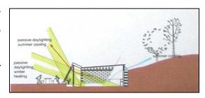
the roof. The locations of these corridors allow for the easy flow of water to and from the appliances and fixtures, as well as ample sunlight for the growth of the plants of the system. The front wall of the Earthship is usually composed of glazing inserted in a wood frame that is clad with steel. This wall may be sloped, or vertical, depending on the location of the dwelling and the desires of the homeowners. The front wall rests on a foundation of packed tires.
