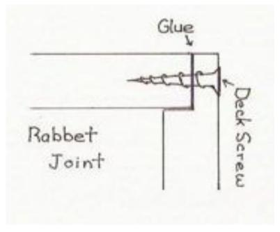
Set your router table so that the router blade is 3/8" above the table and 3/4" out from the fence. This will give you a rabbet ½ way through the end board the width of the side board. Check the setting for your materials as material widths may vary.
