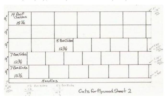
On three of the sheets, there will be a remaining strip a little less than 2 ½" wide. The final sheet will have a remaining strip a little less than 11 ½" wide. If you cut that final strip down to 9" you will have enough for a 29<sup>th</sup> Box and the remaining handles. Mark the actual width in pencil on each strip and set aside.
