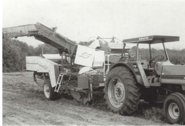
FIGURE 7. A two-row sweet potato combine that does not require vine removal.
