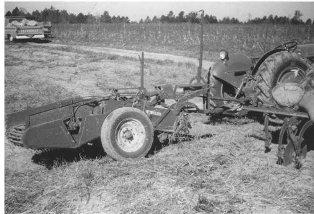
FIGURE 4. A low, flatbed potato digger used to dig sweet potatoes.
