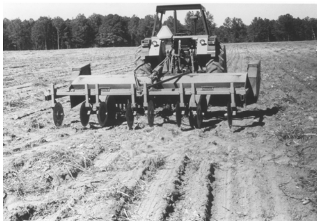
FIGURE 3. A modified flail chopper for vine removal.
