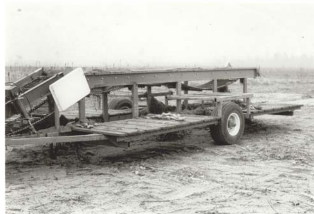
FIGURE 5. A sweet potato harvester using two, rod link, chain conveyors.
