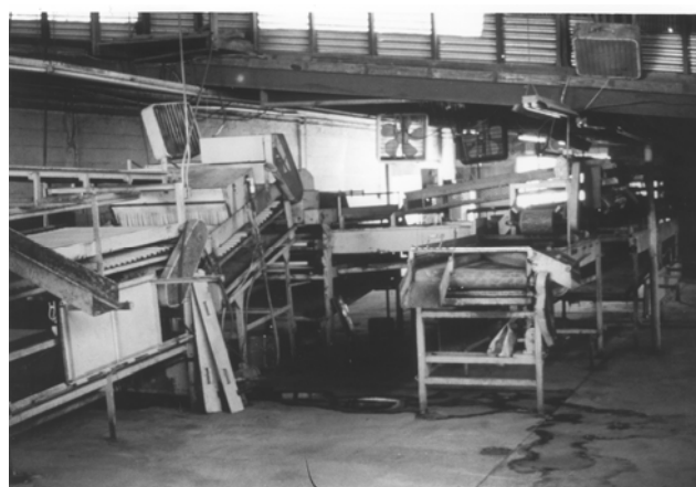
FIGURE 8. Typical washing and grading packing line top-dump tank, bottom-sorting and grading.
