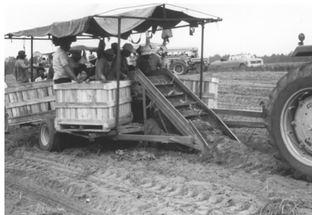
FIGURE 5. A sweet potato harvester using two, rod link, chain conveyors.
