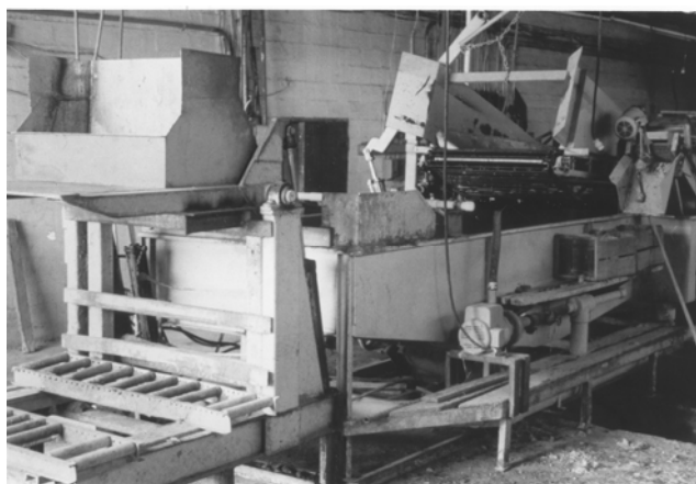
FIGURE 8. Typical washing and grading packing line top-dump tank, bottom-sorting and grading.
