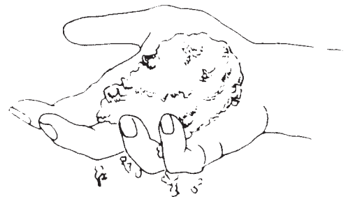
Figure 1. Pick up a handful of soil and roll it into a ball. If the soil sticks together and will not crumble easily, it is too wet to work.
